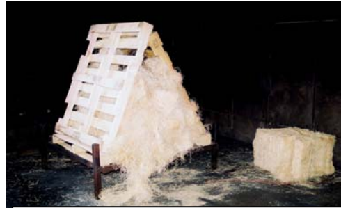
Figure 1 – fuel arrangement (pallets)
